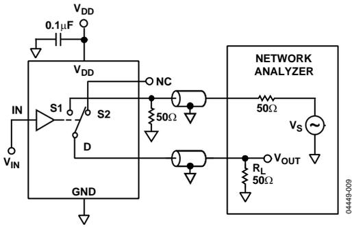
$$\text{OFF ISOLATION} = 20 \text{ LOG } \frac{V_{\text{OUT}}}{V_{\text{S}}}$$
