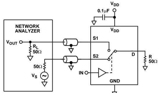
$$\text{CHANNEL-TO-CHANNEL CROSSTALK} = 20 \text{ LOG } \frac{V_{\text{OUT}}}{V_{\text{S}}}$$
