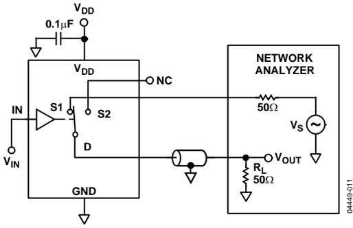
$$\text{INSERTION LOSS} = 20 \text{ LOG } \frac{V_{\text{OUT WITH SWITCH}}}{V_{\text{OUT WITHOUT SWITCH}}}$$
