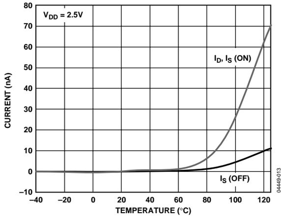
Figure 10. Leakage Current vs. Temperature,  $V_{DD} = 2.5V$
