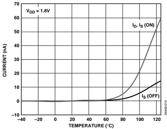
Figure 11. Leakage Current vs. Temperature,  $V_{DD} = 1.8V$
