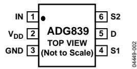
Figure 2. Pin Configuration
