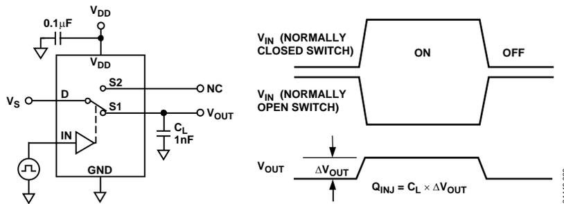
Figure 24. Charge Injection
