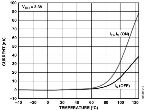
Figure 9. Leakage Current vs. Temperature,  $V_{DD} = 3.3V$
